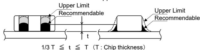
Accordingly increasing the solder volume, the mechanical stress to product is also increased. Excessive solder volume may cause the failure of mechanical or electrical performance.
