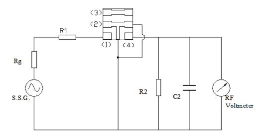
R1=280 $\Omega$  (1±5%,) R2= 330 $\Omega$  (1±5%,) Rg=50 $\Omega$ ; C2=10pF (Including stray capacitance and input capacitance of RF voltmeter), S.S.G: Output Voltmeter; (1): Input; (2): Ground; (3): Float; (4): Output
