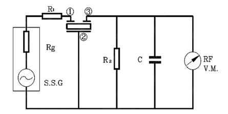
C=10pF(Including stray capacitance and input capacitance of RF voltmeter)
