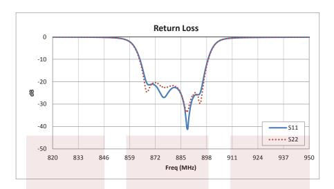
Bandpass Cavity Filter Operating From 869 MHz to 894 MHz With SMA Female Connectors from Fairview Microwave is instock and available to ship same-day. All of our RF/microwave products are available off-the-shelf from our ISO 9001:2008 certified facilities in Allen, Texas. Fairview Microwave is RF on-demand.
