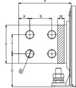
**Note:** all FN3311 and FN3310 provide unsymmetrical mounting hole patterns to prevent inverse filter installation in the field.
