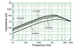
AC Line Filters - Common Mode SS Coils, 11V/H-CH Series
