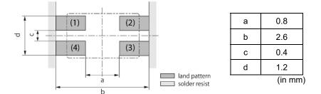
Do not use gilded pattern. A copper wire may cause open by dissolution of metallization.
