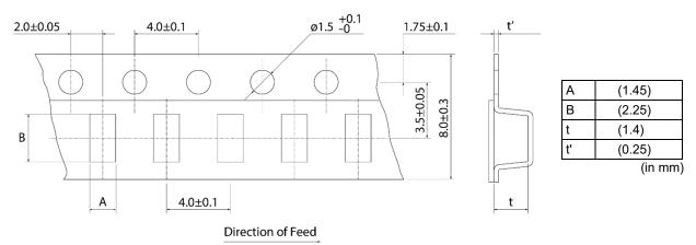
\* The dimensions of the cavity are measured at its bottom.
