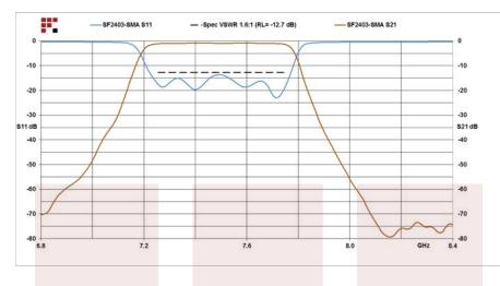
Bandpass Cavity Filter Operating From 7.25 GHz to 7.75 GHz With SMA Female Connectors from Fairview Microwave is instock and available to ship same-day. All of our RF/microwave products are available off-the-shelf from our ISO 9001:2008 certified facilities in Allen, Texas. Fairview Microwave is RF on-demand.
