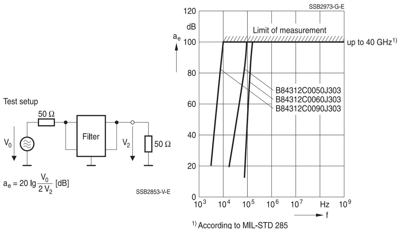
**Filters for control and communication lines with HEMP-Protection**
