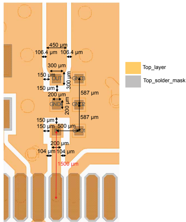
Figure 13. PCB land pattern recommendations
