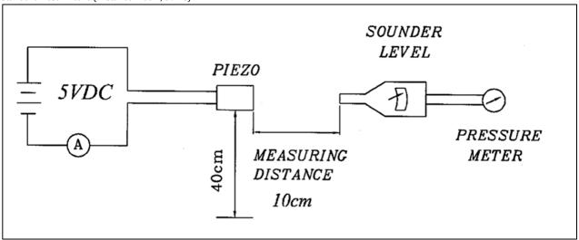
**Reliability Testing** Standard Test Condition (+5~+35°C, 45~85% RH)
