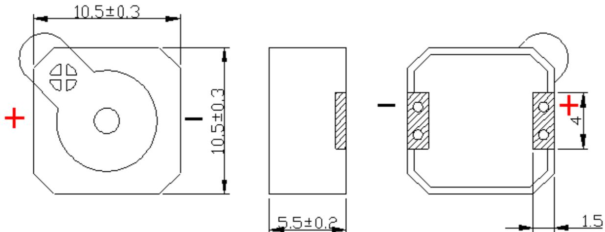
Attention: Must be installed with correct polarity.
