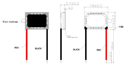
General tolerance = ±0.2 mm and all measurements in mm unless otherwise noted.
