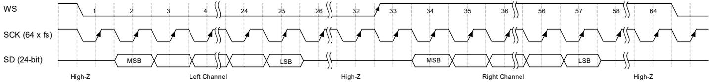
**Figure 25. High Quality Mode Stereo Output I<sup>2</sup>S Format**
