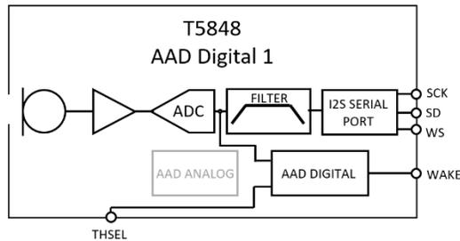
**Figure 15. Block Diagram for AAD Digital 1 Operation**
