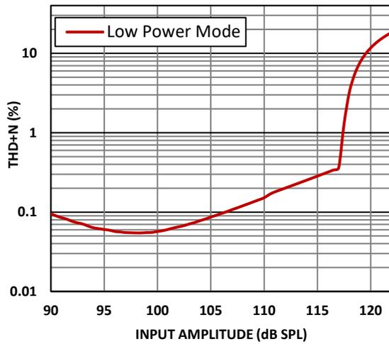
Figure 6. THD + N Low Power Mode – 1 kHz Input
