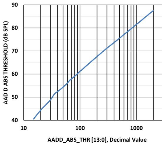
Figure 10. AAD Digital 1,2 Absolute Threshold vs Register Value
