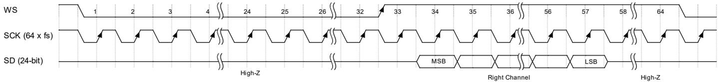
**Figure 27. High Quality Mode Stereo Right Channel (LR = 1)**
