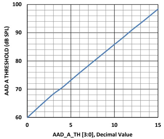
Figure 9. AAD Analog Threshold vs Register Value
