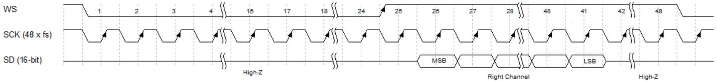
**Figure 30. Low Power Mode Stereo Right Channel (LR = 1)**
