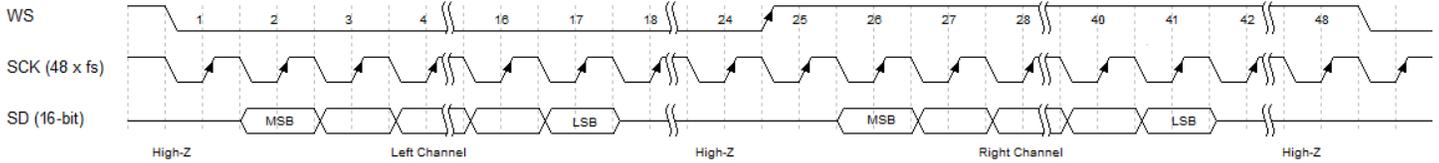
**Figure 28. Low Power Mode Stereo Output I<sup>2</sup>S Format**
