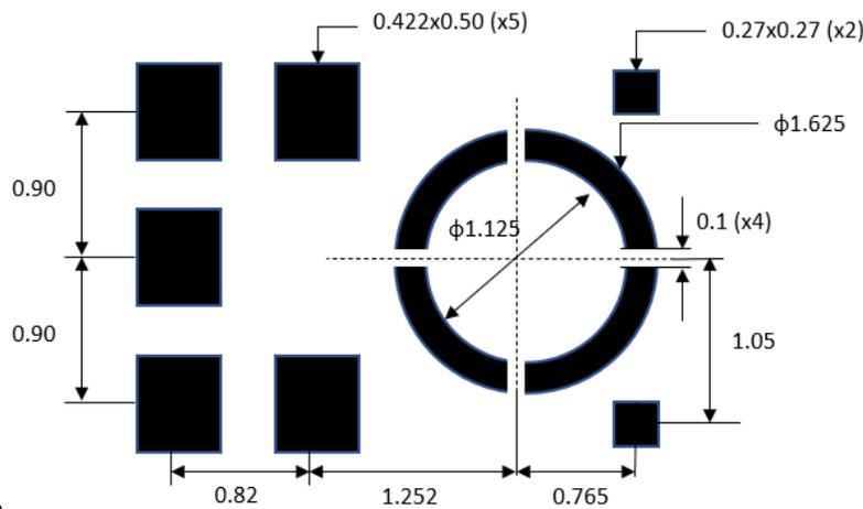
Figure 34. Suggested Solder Paste Stencil Pattern Layout
