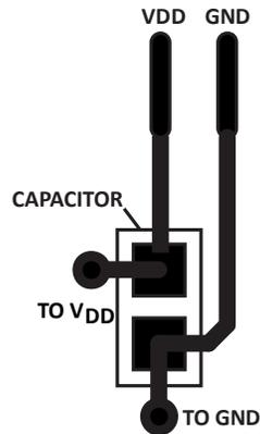
**Figure 32. Recommended Power Supply Bypass Capacitor Layout**
