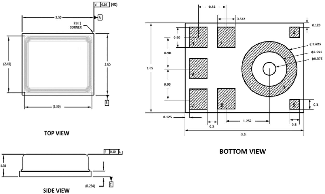
**Figure 35. 8-Terminal Chip Array Small Outline No Lead Cavity [LGA\_CAV]
