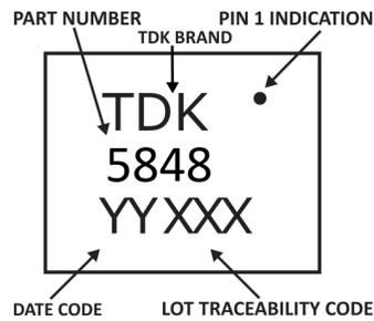
**Figure 36. Package Marking Specification (Top View)**
