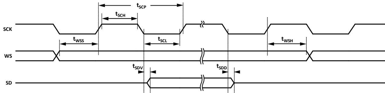
**Figure 1. I<sup>2</sup>S Output Timing**
