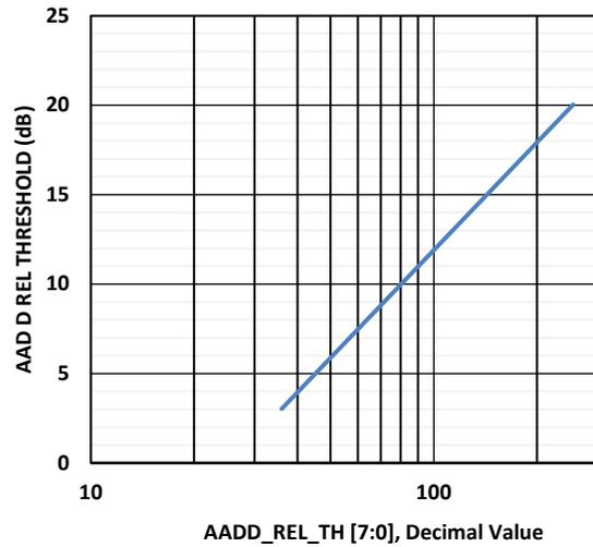
Figure 11. AAD Digital 1,2 Relative Threshold vs Register Value
