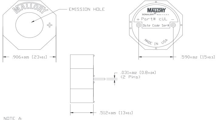
NOTE A: TERMINALS - .031" DIA. NICKEL/TIN COATED BRASS. NOTE R:
