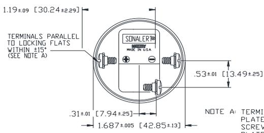
NOTE A: TERMINALS--032 BRASS TIN PLATED, TAPPED FOR #6-32 SCREW. TWO #6-32 NICKEL PLATED BRASS SCREWS INCLUDED. WILL ACCEPT 1/4" QUICK CONNECT.
