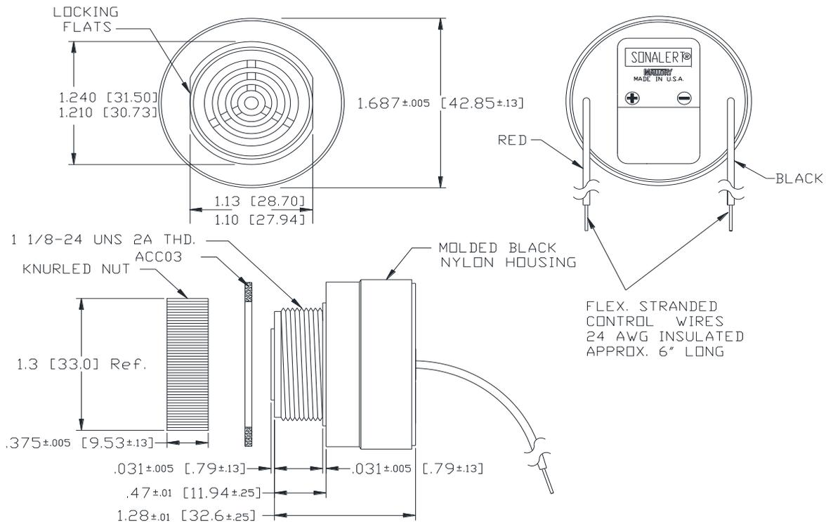
MOUNTING- REMOVE BLACK PLASTIC NUT WHILE LEAVING GASKET ON THREADED NECK OF ALARM. INSERT THREADED NECK THROUGH APPROPRIATE SIZED PANEL HOLE. SCREW NUT BACK ONTO THREADED FRONT SECURING ALARM TO PANEL. MAX RECOMMENDED TORQUE IS 10 IN-LBS.
