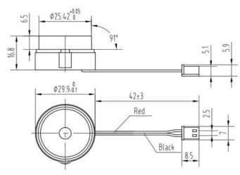
Connector Housing: A2503HOO-2P Connector crimp: A2503TOP-2
