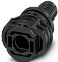
Panel feed-through, Range of articles: Sunclix, Device connector, front mounting, housing material: PPE, color: black, number of positions: 1, min. conductor cross section: 2.5 mm<sup>2</sup>, max. conductor cross section: 6 mm<sup>2</sup>, rated voltage: 1500 V DC, rated current: 38 A, Connection method: Crimp, Type of contact: Pin
