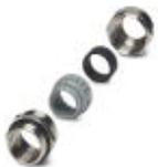
Metal screw connection up to 5 bar, thread length: 6 mm, cable diameter: 11 - 16 mm, WAF 27, screw connection: M20
