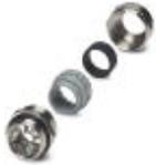
EMC screw connection up to 5 bar, thread length: 5 mm, cable diameter: 7.0 - 12.5 mm, WAF 24, screw connection: M20
