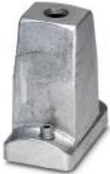
HEAVYCON ADVANCE sleeve housing B6, with high-grade steel screw locking (hexagonal socket-head), salt water resistant aluminum, height 100 mm, with thread, 1xM20, straight cable outlet, without surface; conductive seal (EMC properties)
