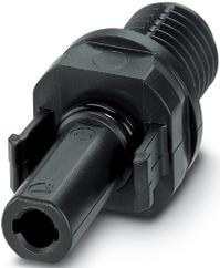
Panel feed-through, Range of articles: Sunclix, Photovoltaic connector, housing material: PPE, color: black, number of positions: 1, rated voltage: 1500, Connection method: Crimp, Type of contact: Socket
