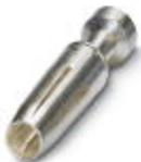
Turned 2.5 crimp contact, individual female contact, core diameter 0.75 to 1.00 mm<sup>2</sup>, silver-plated
