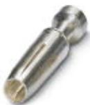
Turned 2.5 crimp contact, individual female contact, core diameter 0.5 mm<sup>2</sup>, silver-plated
