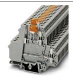
Feed-through terminal block, Connection type: Screw connection, Cross section: 0.2 mm² - 4 mm², AWG: 24 - 12, Nominal current: 26 A, Nominal voltage: 400 V, Length: 80 mm, Width: 6 mm, Color: gray, Assembly: NS 35/7,5, NS 35/15, NS 32
