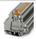
Feed-through terminal block, Connection type: Screw connection, Cross section: 0.2 mm² - 4 mm², AWG: 24 - 12, Nominal current: 26 A, Nominal voltage: 400 V, Length: 80 mm, Width: 6 mm, Color: gray, Assembly: NS 35/7,5, NS 35/15, NS 32
