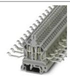
Disconnect and test disconnect terminal block, Connection type: Screw connection, Cross section: 0.2 mm² - 2.5 mm², AWG: 24 - 14, Nominal current: 24 A, Nominal voltage: 500 V, Length: 42.5 mm, Width: 6.2 mm, Color: gray, Assembly: NS 35/7,5, NS 35/15, NS 32
