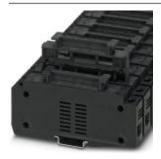
Fuse modular terminal block, Connection method: Screw connection, Cross section: 1.5 mm²- 25 mm², AWG: 18 - 3, Nominal current: 32 A, Nominal voltage: 1500 V, Width: 23 mm, Fuse type: gG / gPV / 10.3 x 85, Mounting type: NS 35/7,5, NS 35/15, Color: black
