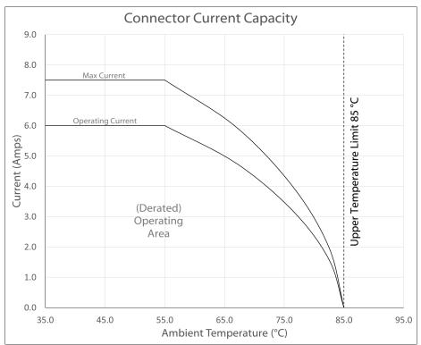
Testing based on IEC 60512-5-2. Max current curve generated with isolated test article under controlled environmental conditions, and does not take into account external factors such as housings, mating cables, or other circuitry. Operating current curve (derated by 20% of maximum values) accounts for external factors, and manufacturing variation.
