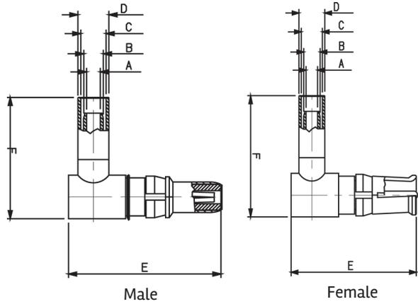
These removable contacts are suitable for the contact cavities of the DMW series and DW series.
