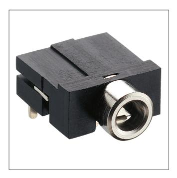
Jack chassis socket, 3.5 mm acc. to JIS C 6560 JC35J3Z, 3 poles/stereo, angular version, with break contact, for printed circuit boards
