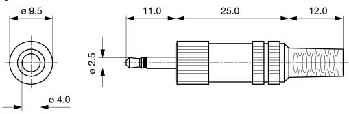
Cable diameter max. 4.0 mm
