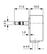
Cable diameter max. 4.0 mm
