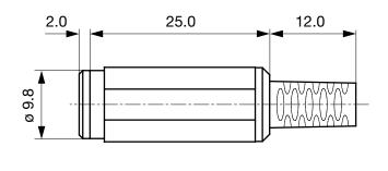
Cable diameter max. 4.0 mm
