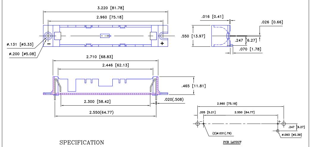
HOLDER: SELF-EXTINGUISHING THERMOPLASTIC POLYSTER PBT, BLACK, UL94V-0 CONTACTS: 301 - 304 SPRING TEMPER STAINLESS STEEL, NICKEL PLATED,
