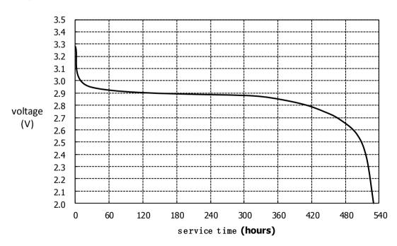
Discharge method:30KΩ, 24 hours/day EV 2.0V temperature of 20±2 $^{\circ}$ C
