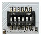
The switch on the right side (marked with ON) codes for a 1, and the switch on the left side codes for a 0. The 4-bit address is decoded:
