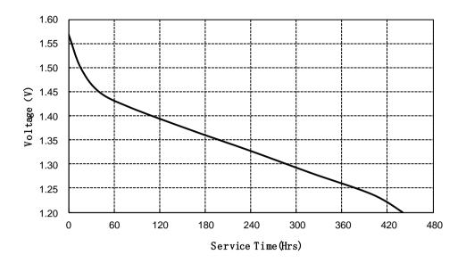
Discharge method: 22k $\Omega$ , 24hours/day, E.V. 0.9V Temperature: 20±2 $^{\circ}$ C
