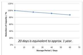
Measurement conditions:Temp:23 deg C Storage conditions: 60 deg C Dry Load:5.1k $\Omega$
