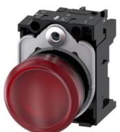
Indicator light, 22 mm, round, plastic, red, lens, smooth, with holder, LED module, with integrated LED 230 V AC, screw terminal, with laser labeling, upper case and lower case, always upper case at beginning of line
