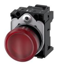
Indicator light, 22 mm, round, plastic, red, lens, smooth, with holder, LED module with integrated LED 110 V AC, spring-type terminal, with laser labeling, upper case and lower case, always upper case at beginning of line
