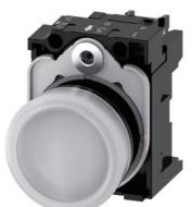
Indicator lights, 22 mm, round, plastic, white, lens, smooth, with holder, LED module, with integrated LED 24 V AC/DC, screw terminal, with laser labeling, inscription or symbol Customer-specific selection with SIRIUS ACT configurator (CIN)
