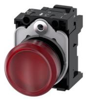
Indicator light, 22 mm, round, plastic, red, lens, smooth, with holder, LED module, with integrated LED 24 V AC/DC, spring-type terminal, with laser labeling, upper case and lower case, always upper case at beginning of line
