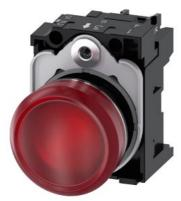
Indicator light, 22 mm, round, metal, shiny, red, lens, smooth, with holder, LED module with integrated LED 24 V AC/DC, screw terminal, with laser labeling, upper case and lower case, always upper case at beginning of line
