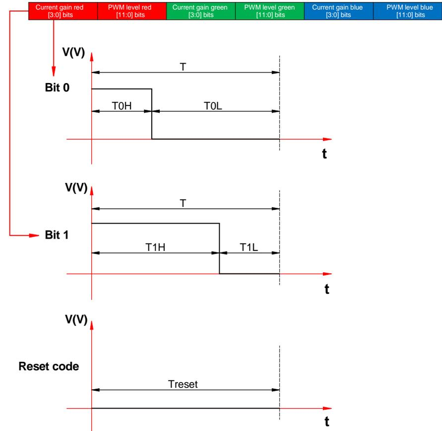
Treset is not to scale. The 48-bit data is formed by red, green and blue data, each with 12-bit PWM and 4-bit current level selector.
