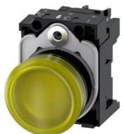
Indicator lights, 22 mm, round, plastic, yellow, lens, smooth, with holder, LED module with integrated LED 110 V AC, screw terminal, with laser labeling, upper case and lower case, always upper case at the beginning of the word
