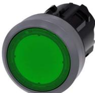
Indicator light in illuminated pushbutton design, 22 mm, round, plastic with metal front ring, green, with laser labeling, upper case and lower case, always upper case at beginning of line
