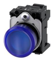
Indicator light, 22 mm, round, plastic, blue, lens, smooth, with holder, LED module, with integrated LED 230 V AC, spring-type terminal, with laser labeling, upper case and lower case, always upper case at beginning of line
