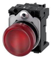
Indicator lights, 22 mm, round, metal, shiny, red, lens, smooth, with holder, LED module with integrated LED 24 V AC/DC, screw terminal, with laser labeling, upper case
