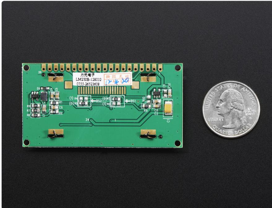
Getting started is easy! [We have a detailed tutorial and example code in the form of an Arduino library for text and graphics. \(https://adafru.it/j6a\)](https://adafru.it/j6a) You'll need a microcontroller with more than 512 bytes of RAM since the display must be buffered. The library can print text, bitmaps, pixels, rectangles, circles and lines. It uses 512 bytes of RAM since it needs to buffer the entire display but its very fast! The code is simple to adapt to any other microcontroller.
