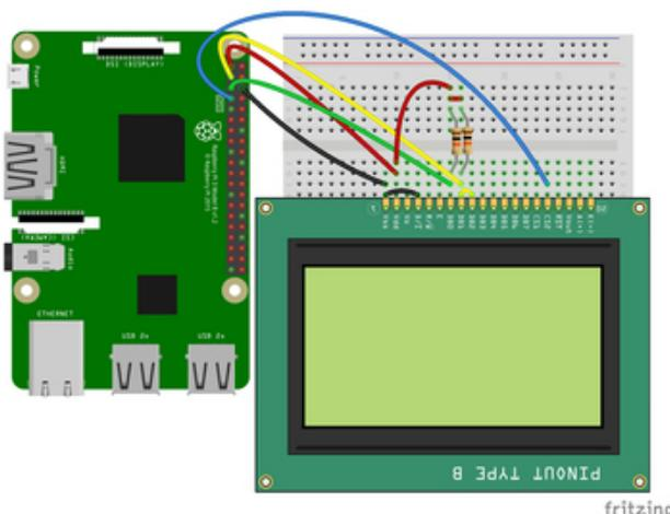
OLED Pin #1 to Raspberry Pi GND
