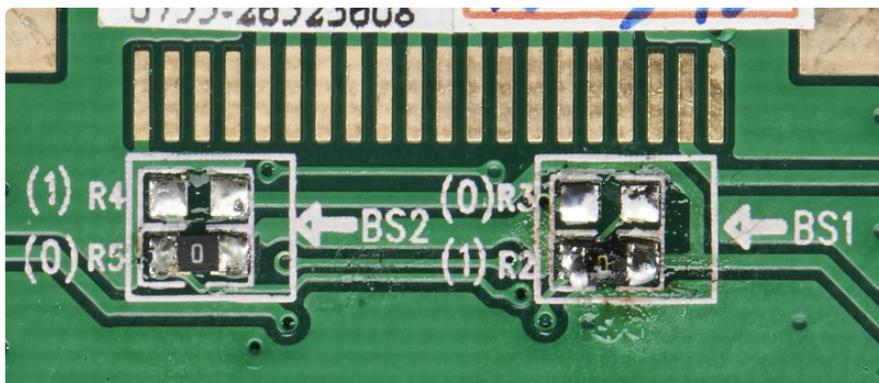
(If you solder and re-solder the resistors 10 times like I did while figuring out all the setting and wiring, you'll get a kinda messy/fluxy look like the above! In that case you can clean up with some IPA wipes. Or just revel in your punk soldering job)
