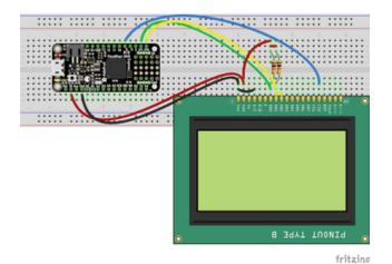
OLED Pin #1 to Microcontroller GND
