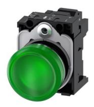
Indicator lights, 22 mm, round, metal, shiny, green, lens, smooth, with holder, LED module with integrated LED 24 V AC/DC, spring-type terminal, with laser labeling, lower case
